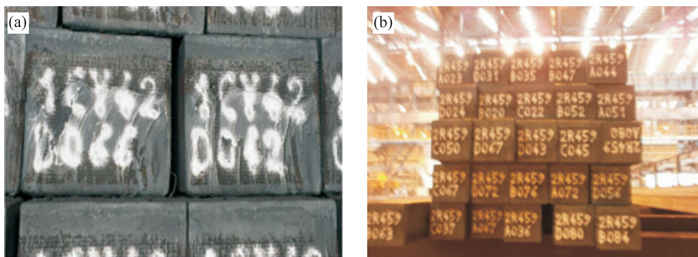
Fig.4. (a) Markings on the blooms before and (b) after improvement.
